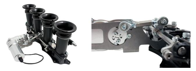
The linkage assembly supplied has been specifically designed to operate AT Power throttles, giving full 360 degrees of rotational positioning and fine adjustment.
